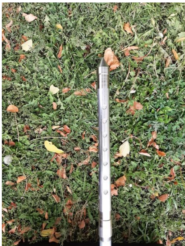
Photo 12: Mini-Piezometer Screen Tip (Photo Date: 2021-09-28)
