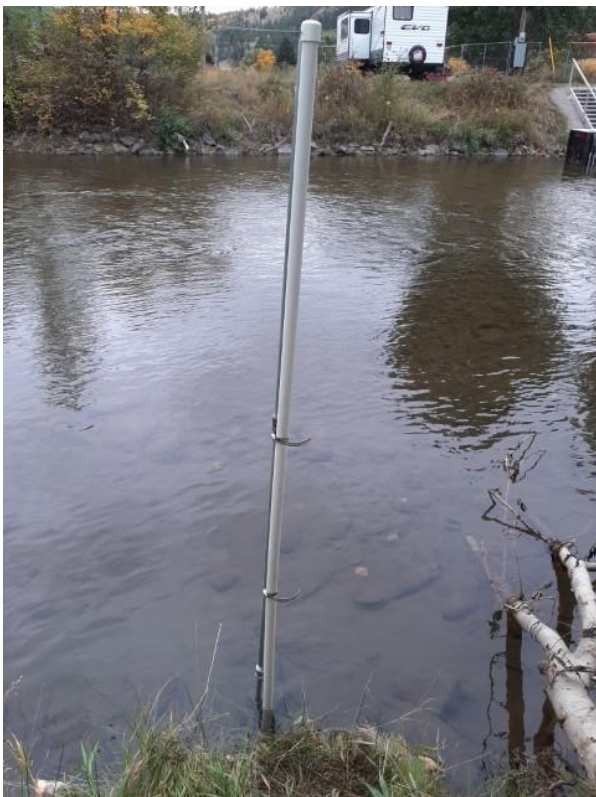
Photo 4: Coldwater River at Voght Park Mini-Piezometer (Photo Date: 2021-09-29)
