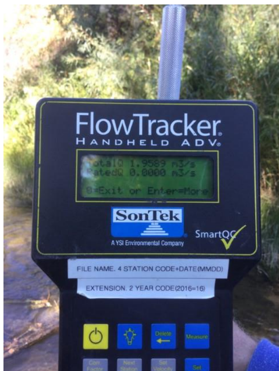
Photo 22: Streamflow Meter (Photo Date: 2021-09-15)
